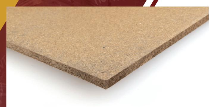
Made of compressed wood fibres from Norwegian Spruce and impregnated with Bitumen Emulsion, Expansion Joint Filler Board is used in the construction of concrete slabs and walls, and as a protection board for waterproofing membranes.
